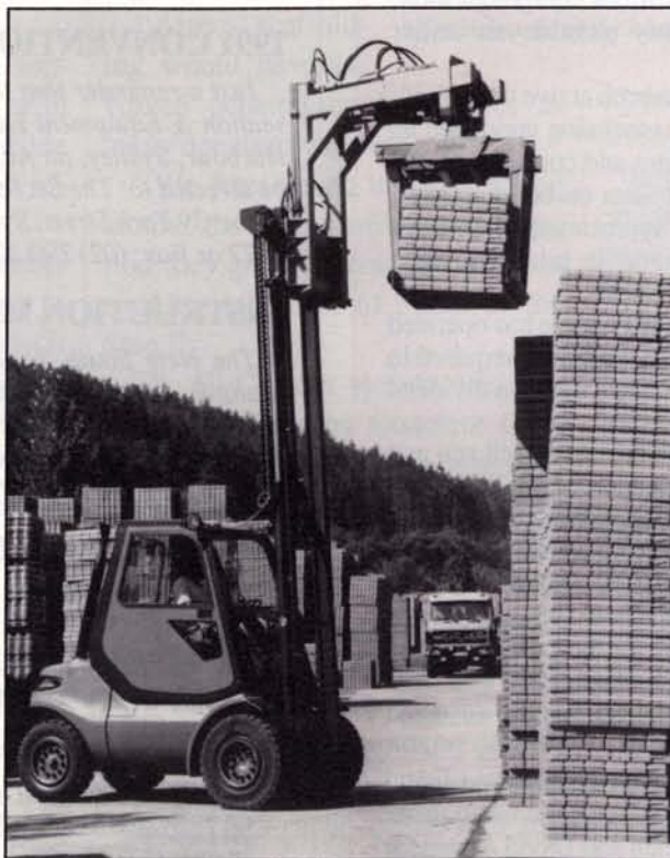
Composite blocks released from production, are stacked by the Linde H45 to a height of 5 metres.
